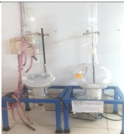
Name of the Instrument: Double Distillation Unit Model No.: 2063/200
