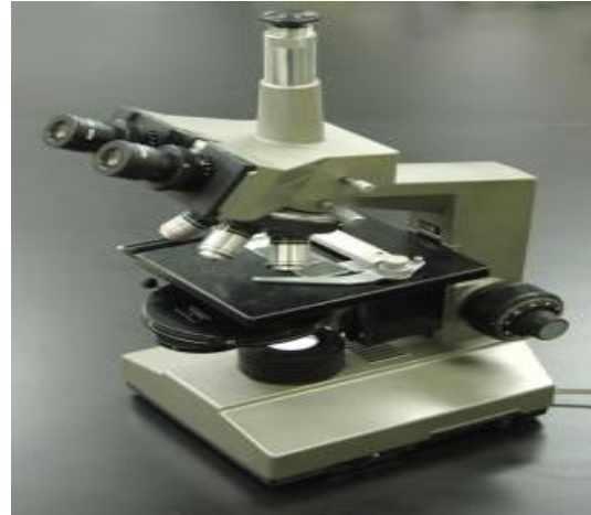
Name of the Instrument: Phase Contrast Microscope Company Name: Magnus MLX-B Plus
